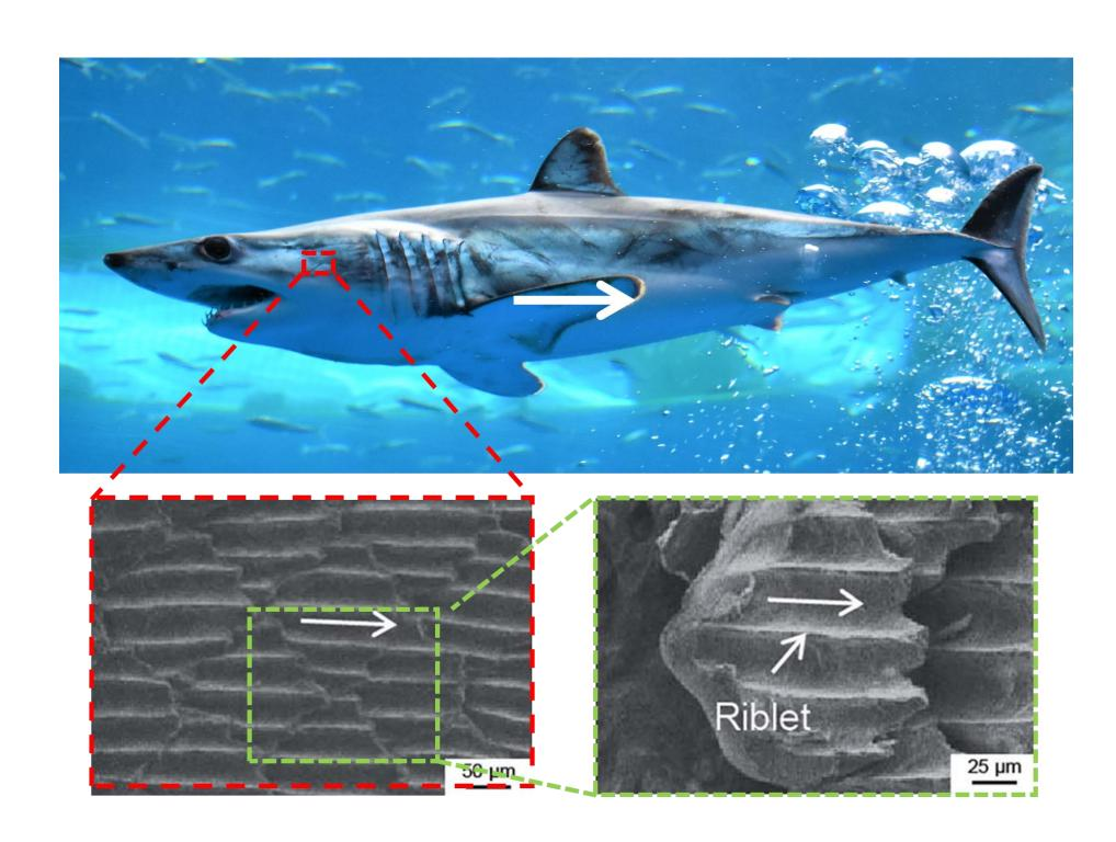
The riblet structures on the skin of fast swimming sharks reduce skin friction drag in the turbulent flow regime allowing them to swim faster.
