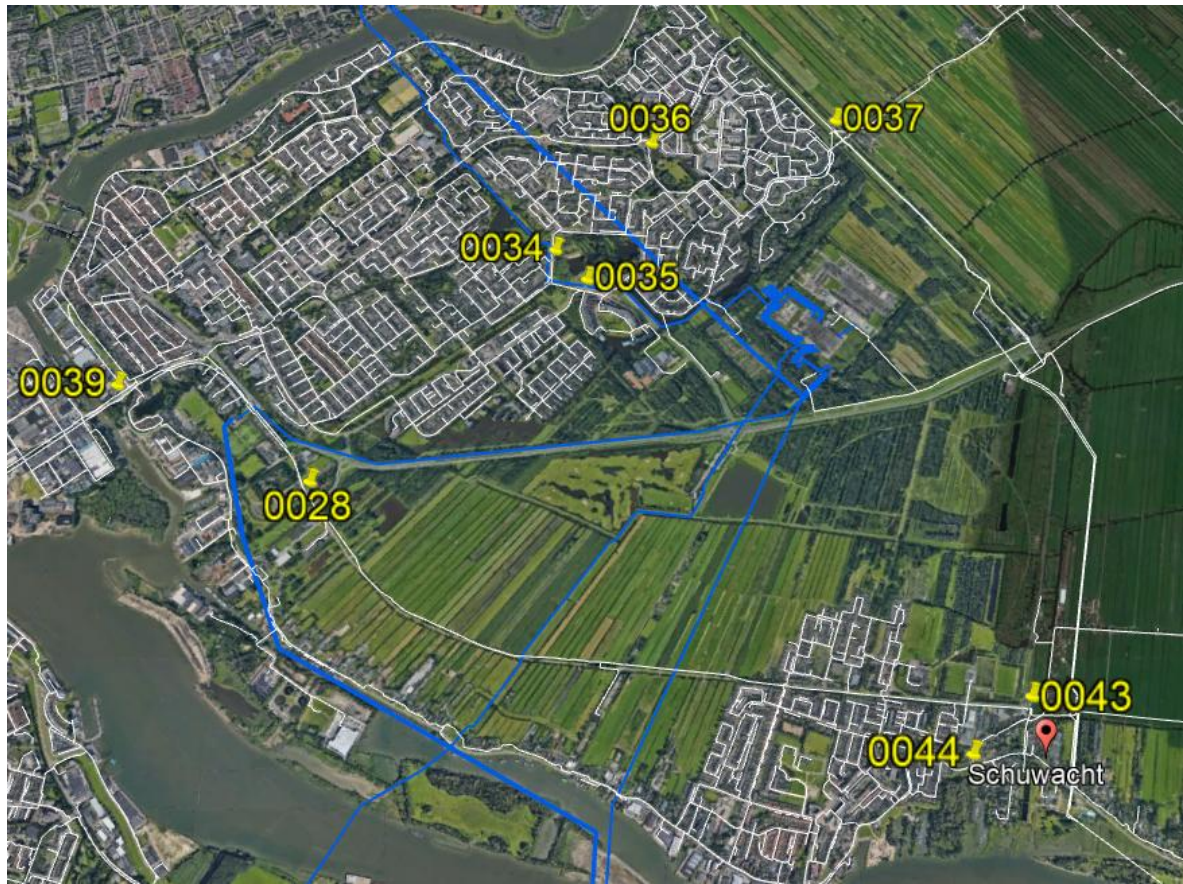
Figure 2 Overview of the eight measurement locations in Krimpen aan den IJssel and Krimpen aan de Lek. In white the drinking water pipes, in yellow the ID's of the corresponding DMAs: 0028, 0034 - 0037, 0039, 0043 and 0044), in blue the high voltage cables, the red pointer is the treatment plant Schuwacht.
